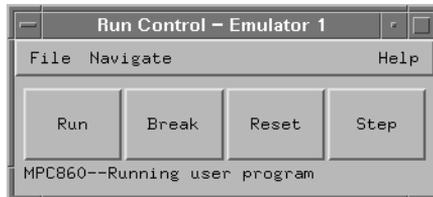
Resetting the processor starts it from a known state. Breaking puts the processor into the background monitor and allows the emulation module to read the microprocessor’s configuration registers (whose contents enable breakpoints among other things).
