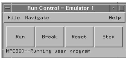
Resetting the processor starts it from a known state. Breaking puts the processor into the background monitor and allows the
