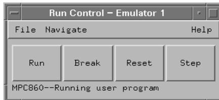
Resetting the processor starts it from a known state. Breaking puts the processor into the background monitor and allows the emulation module to read the microprocessor’s configuration
