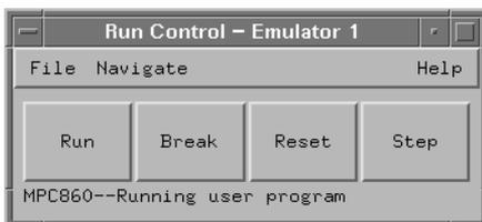
Resetting the processor starts it from a known state. Breaking puts the processor into the background monitor and allows the emulation module to read the microprocessor’s configuration registers (whose contents enable breakpoints among other things).
